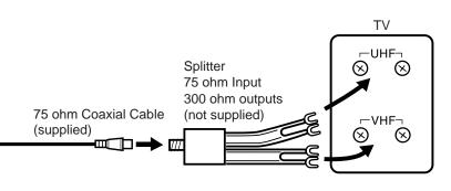
NOTE: If a VHF or UHF antenna is used, set the TV/CATV menu option to the "TV" mode.
